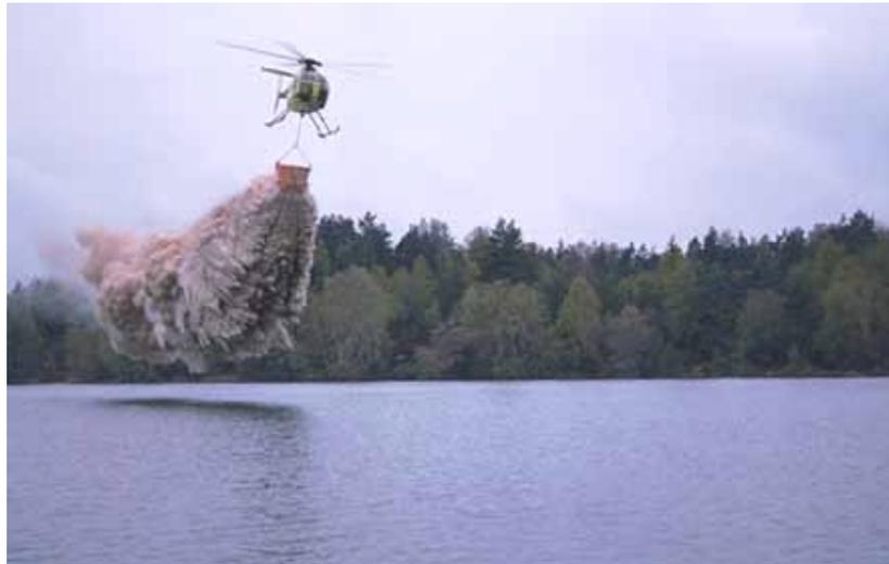
**Figure 2:** Lake liming as a measure to reduce acidity in aquatic ecosystems.
